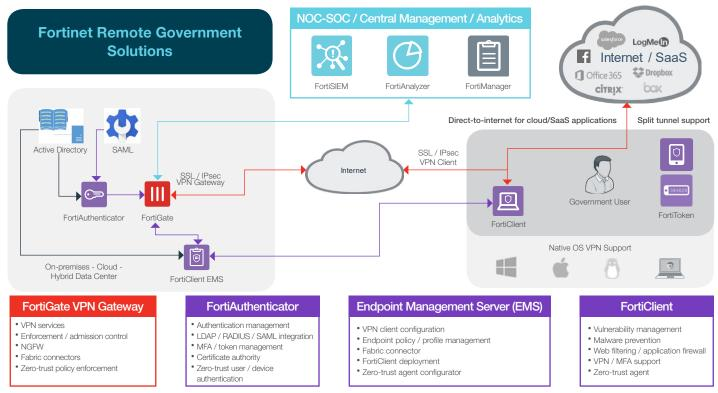
Figure 1: Fortinet solution deployment for standard government worker.
